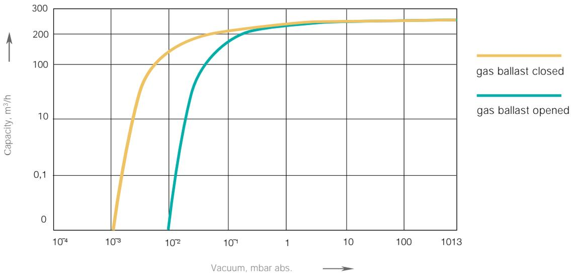
The given data are referred to dry air at the temperature of 20°C, at the atmospheric discharge pressure (1013 mbar). Performances tolerance ±10%.
