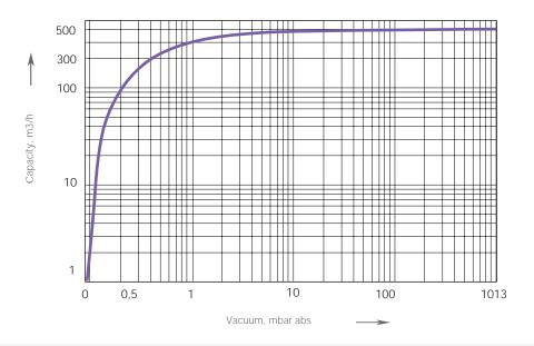
The presented characteristics are valid for dry air at temperatures up to 40  $^{\circ}$ C and an atmospheric pressure of 1013 mbar abs. Tolerance of the characteristics is ± 10%.
